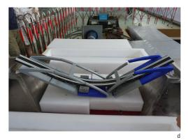
The arrangement of spring elements and the associated decoupling of the superstructure from the abutments significantly reduced the stress. Although the preparation was very time consuming and there were many problems with the implementation, the competition came to a successful end and we left the competition with a positive feeling.
